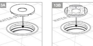
13A. Set the drain receiver in the upright position for standard drain.
