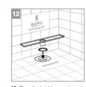
12. Place the height support ring to allow adjust of the drain height. The height may vary depending on the tile thickness.
