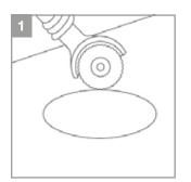
1. Position the tray marking the drain position. Drill a 7 1/2" hole.
