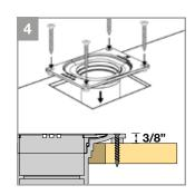
4. Screw the drainbody to the substrate and check the height 3/8". View heights in page 19.
