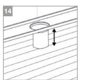
14. Adjust the height of the drain depending on the tile thickness.
