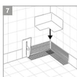
6. Waterproof the walls either with 7. Use the preformed W-S Corners to WATER-STOP membrane or W-S seal the installation laying it and press BOARD. Connect waterproofing fixing firmly. Remove any trapped air to overlapping to walls and curb applying guarantee full adhesión by spreading thin set cement between both parts. the adhesive from the inside out.
