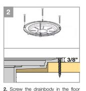
with drive head screws non les than 4 mm (T20). View heights in page 18. Note: In concrete installations set the drain levelled with thinset.
