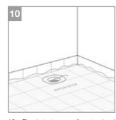
10. Flood test according to local code. If W-S Sealant has been used to install the corners, the test can be performed after 1 hour.
