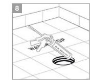
8. Lift the Edge of the WATER-STOP sheet, insert the cannula od the W-S SEALANT and apply a continuous line of W-S SEALANT in the perimeter sealant area.
