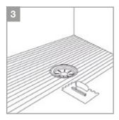
3. Apply thin set cement (tile adhesive) in the drain shower area with 1/4" x 1/4" notched trowel from the shower perimeter to the drain.
