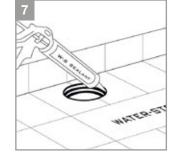
7. Lift the edge of the WATER-STOP sheet, insert the cannula of the W-S Sealant 1/2" and apply a continuous line of mastic in the connection drainbody - WATER-STOP.
