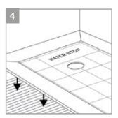
4. Set the W-S HEAVY DUTY SHOWER TRAY in top of the thin set before it cures and apply presure on
