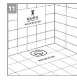
11. Waterproof the walls either with WATER-STOP sheet or W-S Board.
