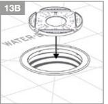
10. Place the bonding flange in top of
