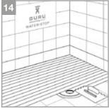
14. Tile on top of the WATER-STOP membrane using the tile required notched trowel
