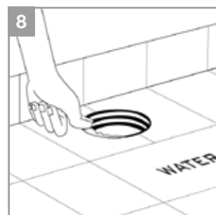
8. Press by hand to distribute the W-S Sealant and clean the excess material on the edge.
