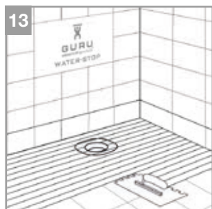
13. Tile on top of the HEAVY DUTY SHOWER TRAY using the tile required notched trowel.
