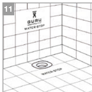
11. Waterproof the walls either with WATER-STOP sheet or W-S Board.
