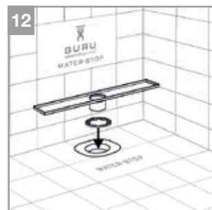
12. Place the height support ring to allow adjustment of the drain height. The height may vary depending on the tile thickness.
